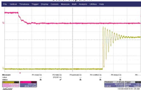
Plot 6 – Switching Time ON Scale: 0.5 \mu\text{s} /Div.
