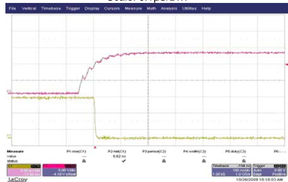
Plot 7 – Switching Time OFF Scale: 0.1 \mu\text{s} /Div.
