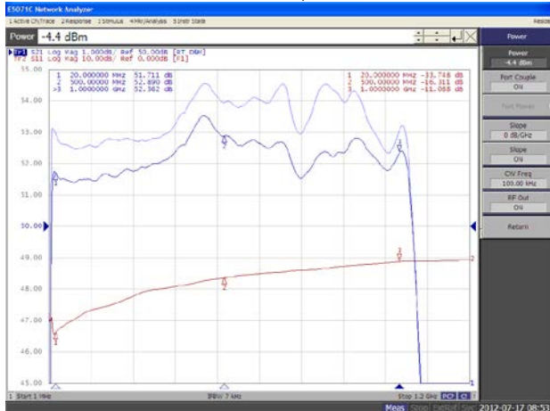
Plot 3 – Gain Adjustment Range @ P_{IN} = -20dBm
